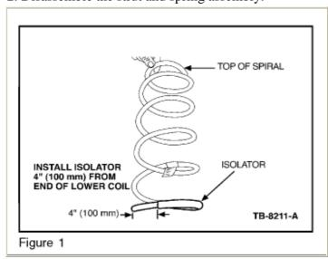
3. If the springs do not have a rubber isolator on the bottom spring coil, install isolators. Clean off any dirt prior to installing the isolator. The isolator should be installed 4" (100 mm) from the end of the coil (Figure 1).
