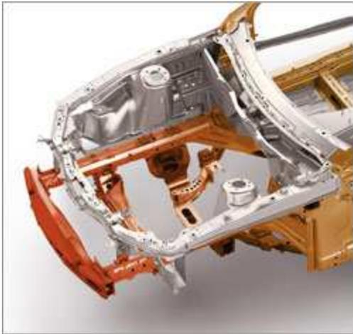
*Engineered from the beginning as both a coupe and convertible, the 2005 Mustang provides torsional rigidity and a stiff chassis for crisper handling at all speeds.*
