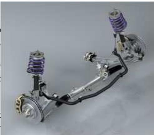
The 2005 Mustang convertible with the chassis MacPherson strut front suspension and torsion bar rear axle designs to their ultimate executions. The result is great driving dynamics with signature, straight-line Mustang performance. This is a direct benefit of the reverse L-configuration of the control arms.
