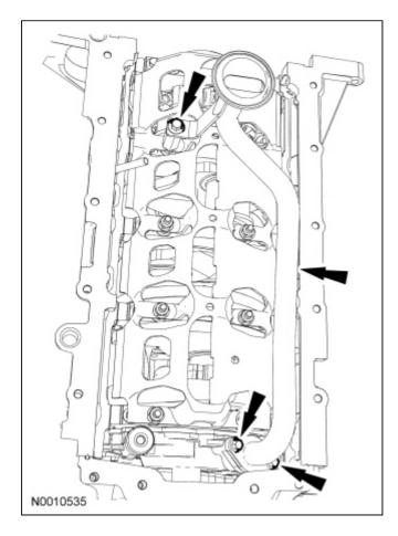
2. Install the oil pan. For additional information, refer to <u>Engine Lubrication Components — Exploded View</u> and <u>Oil Pan in this section</u>.
