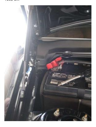
Using a standard Phillips screwdriver, carefully unscrew the plastic screw pin. Once unscrewed, pull up on the retaining pin. 2 places.
