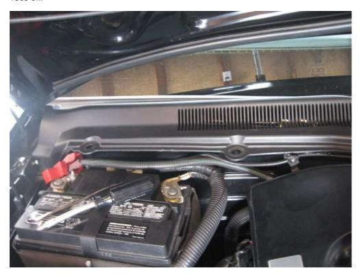
Make sure the cover is positioned back into the original location. The cover seal should sit flush up against the windshield.
