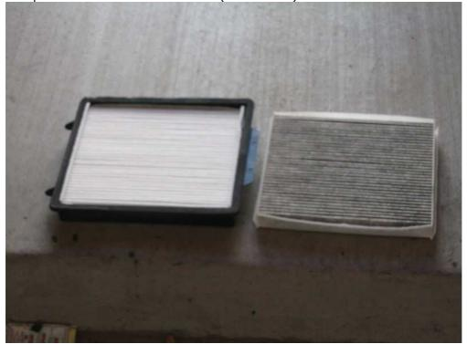
After transferring the black frame from the old filter to the new filter, re-install in reverse order.
